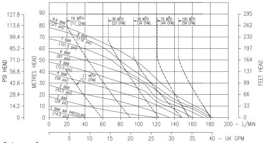
B2505 Metallic Pump, Performance Curve, based on water at ambient temperature
