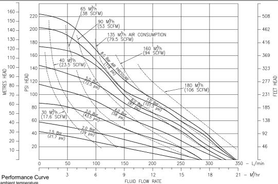
B50 Full Flow 2:1 Pump Performance Curve Performance based on water at ambient temperature
