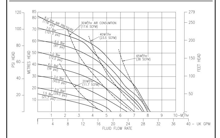
B25 / X25 Hygienic Performance Curve Performance based on water at ambient temperature
