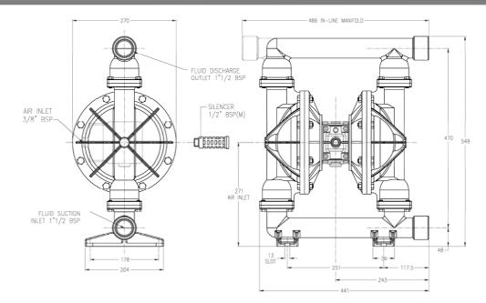
General Assembly :-B4005 Aluminium Pump All dimensions +/- 3mm
